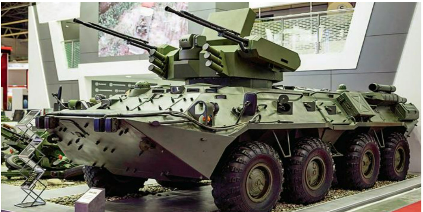
Figure 2. ZAK-23E counter-UAV anti-aircraft system mounted on BTR-82
