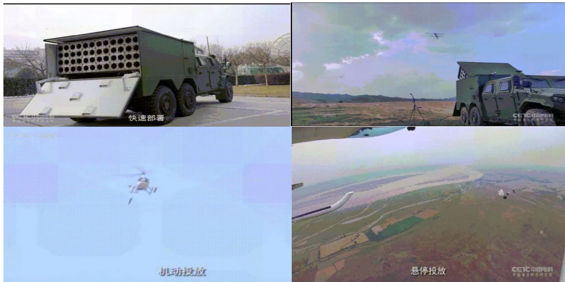
Figure 2. Fixed-wing drone swarm test of land- and air-launched platforms
