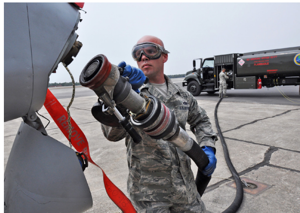
On 25 March 2010, the Air Force fueled and flew this A-10C Thunderbolt II with a 50/50 blend of bio-derived and conventional jet fuel, making it the first military or civilian aircraft to fly with biofuels powering each engine. Courtesy of the U.S. Air Force, photo by Samuel King, Jr.
