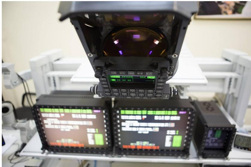
The system combines many of the previously separate informational channels within the aircraft into a single system designed to combine and automate information and then streamline it to pilots in order to give them greater situational awareness. The system provides “intellectual support” for the pilot through its own target acquisition, orienting the aircraft relative to the target and preparing its weapons systems to engage.
