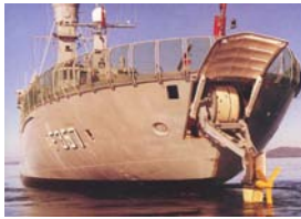
Thetis – sonar is operated from under the deck
