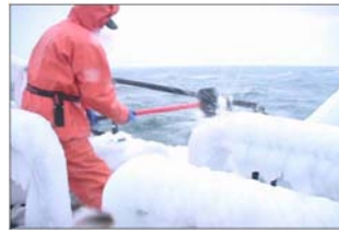
Superstructure icing can affect stability
