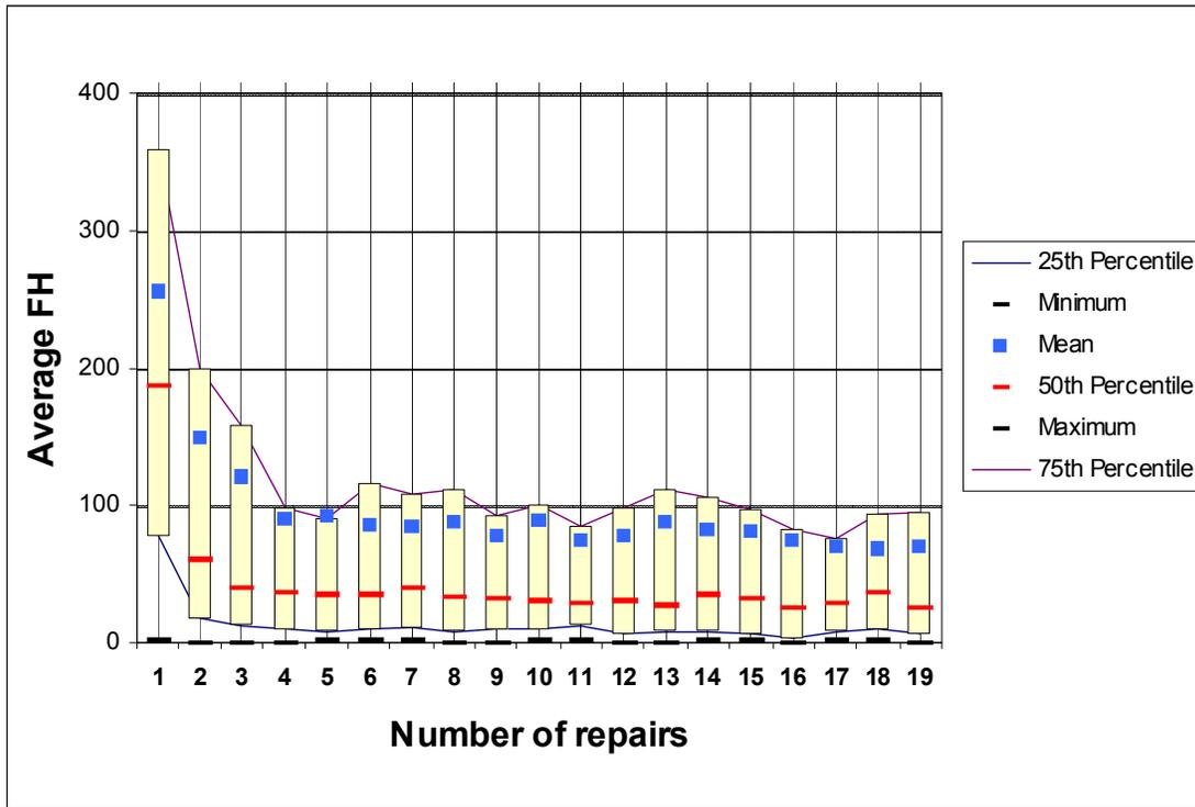
a. Although we only report on a few repair cycles in this graph, for some parts we observe up to 40 cycles. We do not include all of them here because the sample sizes for higher numbers of repair cycles became small and, thus, produced spurious results.
