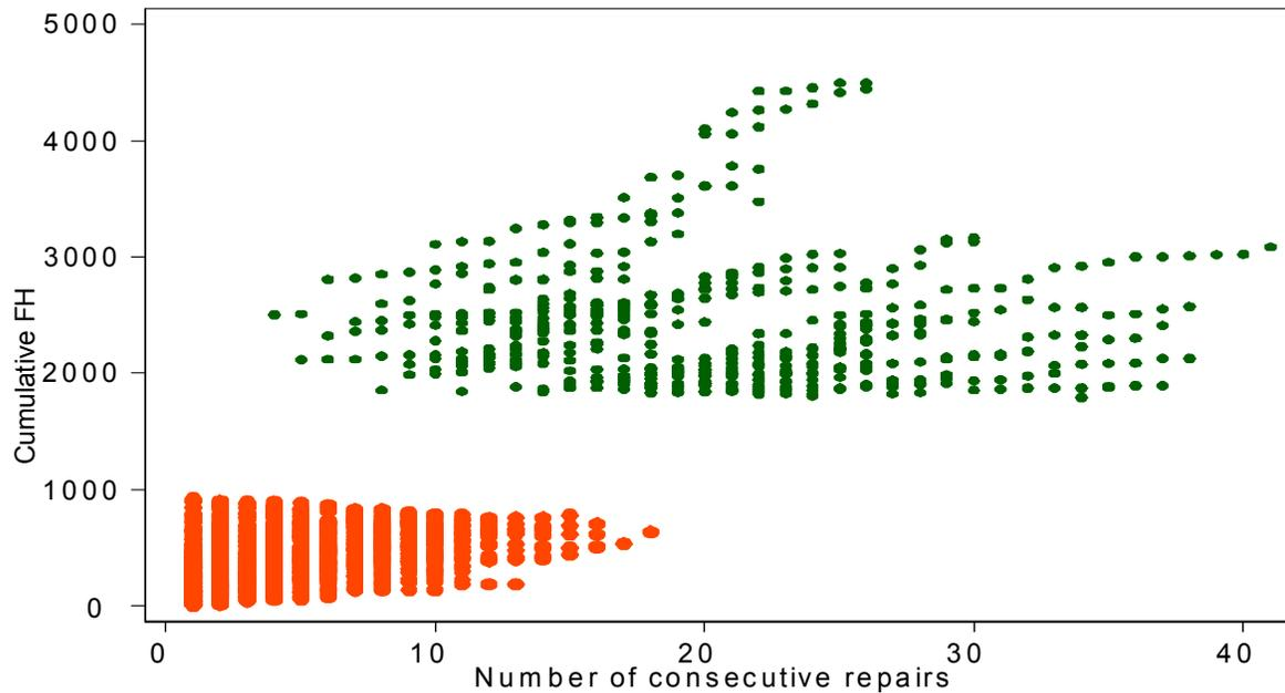
The analysis shows a clear distinction between the parts that provide a relatively large number of FH with a relatively low number of repairs. These would be the *peaches*, which are shown in green. The *lemons* have few cumulative FH and a large number of repairs. They are shown in red.
