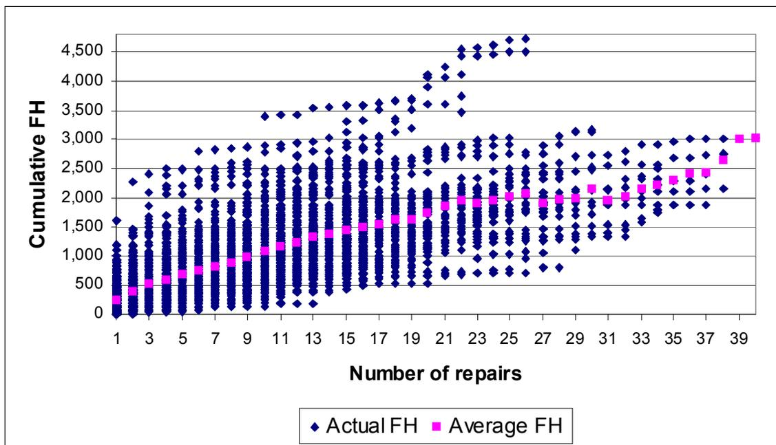
Note that beyond the 20th repair, the sample sizes become smaller (less blue dots) and the trends in the average become more erratic. Also note the wide distribution of FH around the mean.
