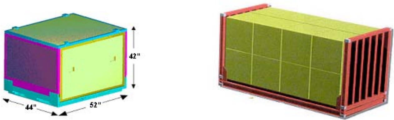
Figure 5. Individual JMIC (left) and 16-interlocked JMICS forming a TEU equivalent (right) 36 (not to scale)
