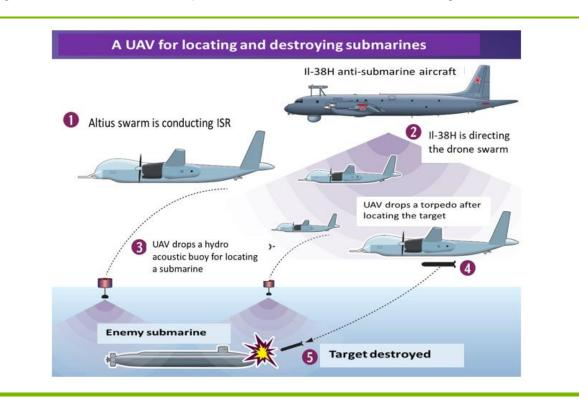
Figure 29. Translated Russian depiction of new anti-submarine drone configuration
